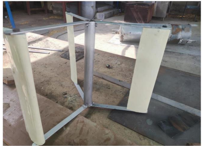
Figure.4. Fabrication of blades, Arms and Rotor Shaft
