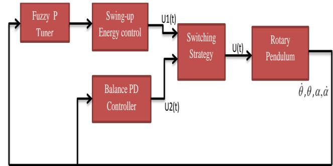
Figure.4. Block Diagram of Swing up Controller [4].
