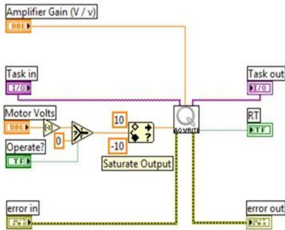
Figure 11. Voltage signal for DC motor Lab-View model.
