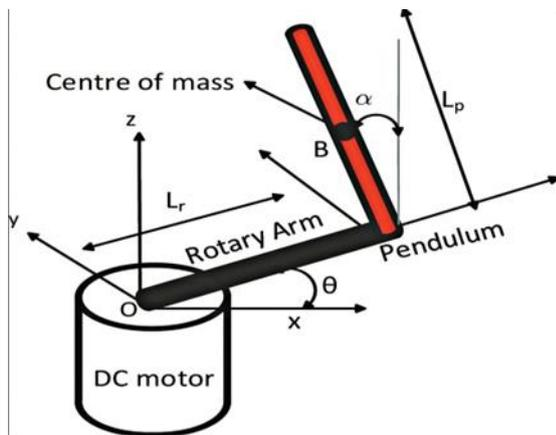
Figure.1. Block Diagram of Inverted Pendulum [5].
