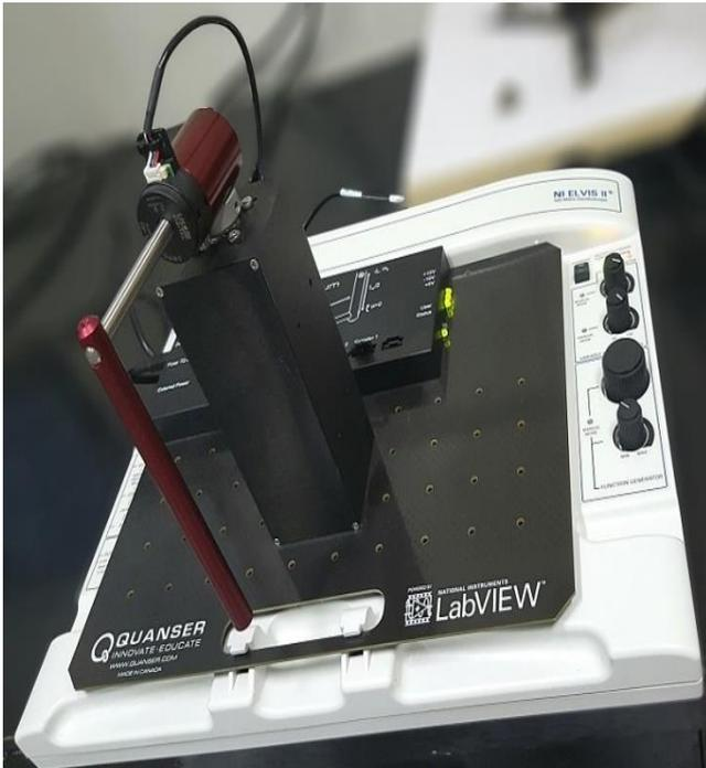
Figure 6. Rotary Inverted Pendulum Kit.
