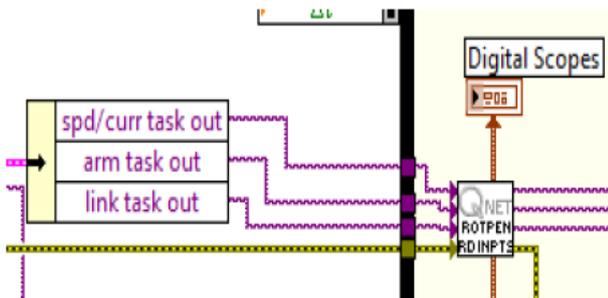
Figure 7. Reading Sensor Data in Lab-view.
