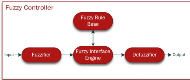
Figure.3. Block Diagram of Fuzzy Logic [12].
