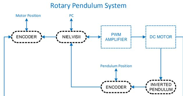
Figure.5. Rotary Pendulum System [5].
