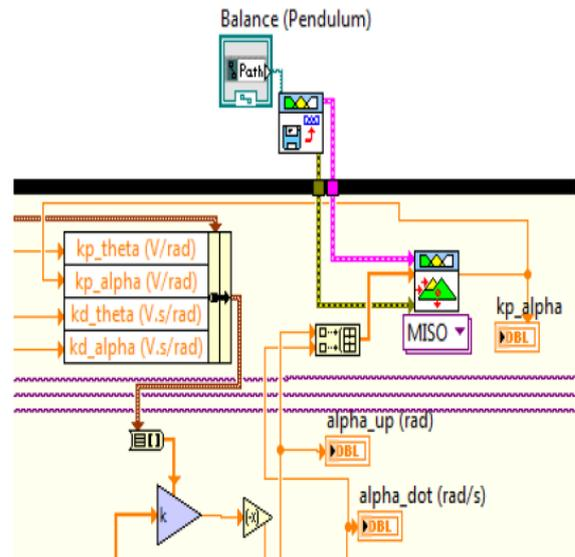
Figure 9. Balance Control in Lab-view.
