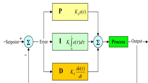
Figure.2. Block Diagram of PID Controller [8].
