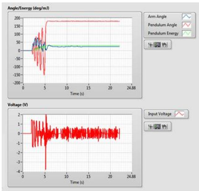
Figure.15. Model Output with PD controller.
