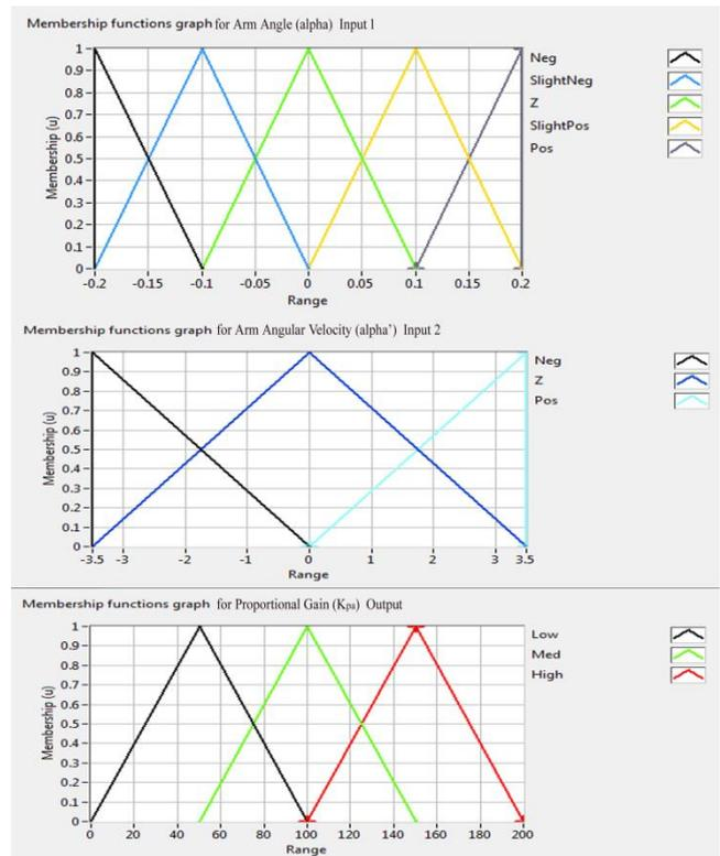
Figure.14. Fuzzy input/output for Balancing Model.
