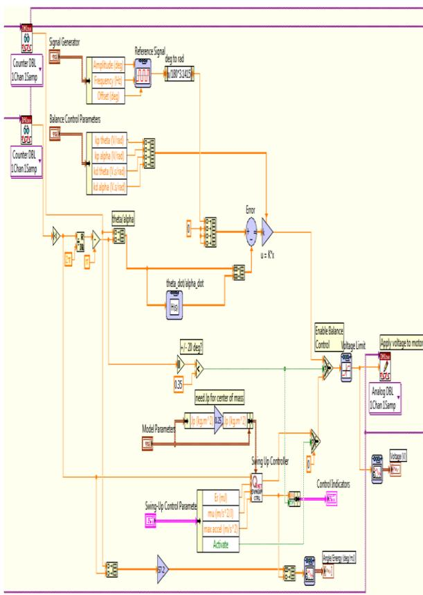
Figure.12. PD Controller in Lab-view
