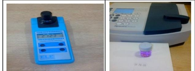
Figure 2. Performing hardness and turbidity test through digital equipment
